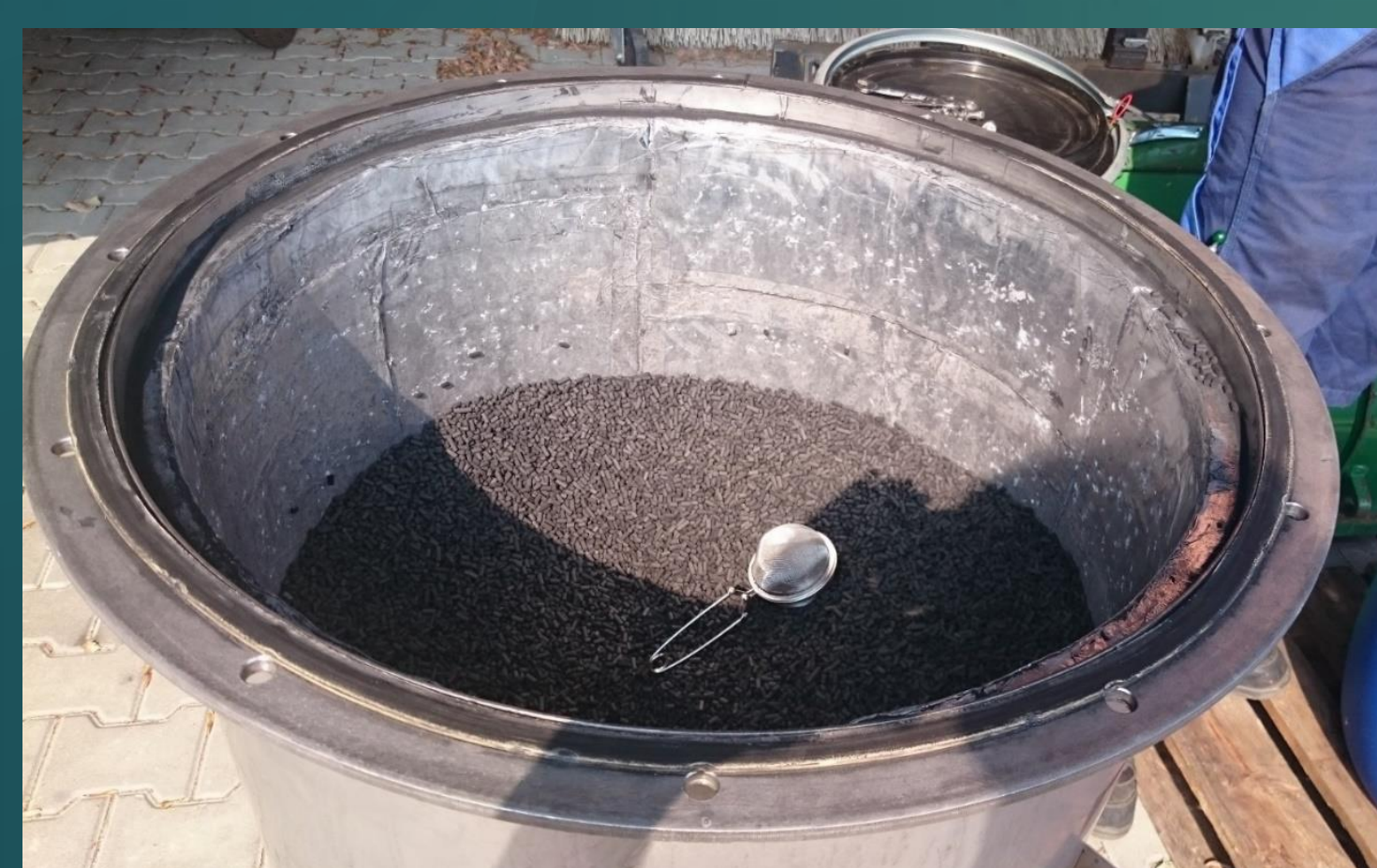
Picture 1: Sampling of coal with a tea egg of an open adsorber
